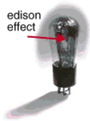
In his rectifying vacuum tube, electrons flow from the negatively charged cathode to the positively charged anode. As the current within the tube is moving from negative to positive, the oscillations of incoming signal are rectified into detectable direct current.
