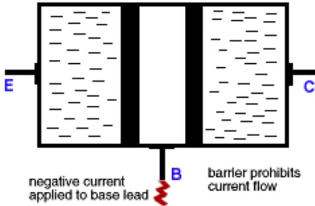
This shows the transistor effect as the transistor is made to alter its state from a starting condition of conductivity (switched 'on', full current flow) to a final condition of insulation (switched 'off', no current flow).
