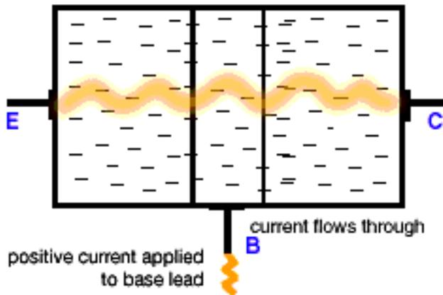
This animation shows the transistor effect as the transistor is made to alter its state from a starting condition of insulation (switched 'off', no current flow) to a final condition of conductivity (switched 'on', full current flow).
