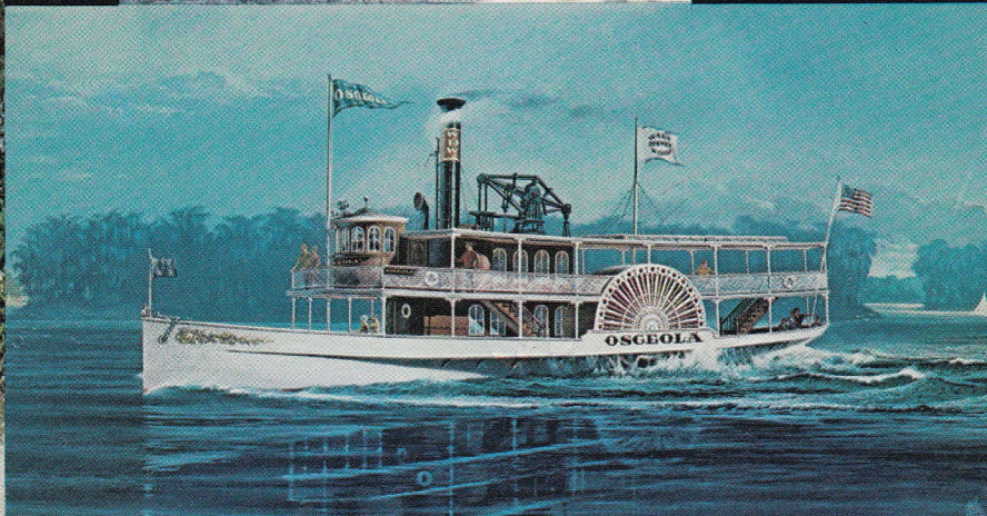
The Osceola will be one of two side-wheel steamboats which will be sailing at Walt Disney World's new Vacation Kingdom at Orlando, Fla. Based on 19th century design, it is the first ship of its kind ever built with fiberglass hull. The Osceola was built by Beatrice's Morgan Yacht Division. (Photo Courtesy Walt Disney Productions.)
