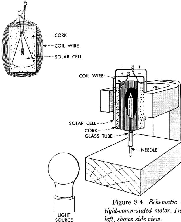
Figure 8-4. Schematic drawing of light-commutated motor. Insert, upper left, shows side view.
